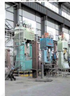
常州精棱订购国内首台最大的125KJ 数控锤整机装配现场 Assembling Site of 125KJ CNC Hammer for Changzhou Jingleng
