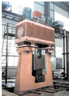
江苏昆山凯诺80KJ数控锤 正在调试 80KJ CNC Hammer for Jiangsu Kunshan Kainuo
