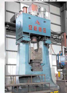
销往文登威力31.5KJ数控锤正在调试 31.5KJ CNC Hammer for Wendeng Weili
